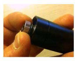
8. Thread the focusing ring, lens assembly and lens spring assembled in step 7 about halfway into the diode module. Final focusing adjustment will be completed later. **Reminder:** The **solid slotted end** of the lens assembly faces **away** from the diode. If the lens is installed backwards, the laser dot will have a "bowtie" shape.
