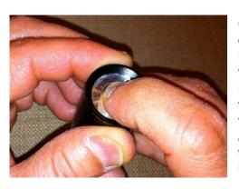
6. Place the bezel/retaining ring over the exposed end of the heat sink. Press the heat sink down with your finger and thread the retaining ring onto the heat sink holder until fully seated. **CAUTION:** Do not touch the diode inside the module with your fingers, and do not let the heat sink rotate as you tighten the bezel/retaining ring. If the heat sink rotates during tightening it could break the wires or pull them off the diode.
