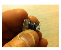
7. If necessary, remove any protective wrapping from the glass lens assembly. Thread the **solid slotted end** of the lens assembly into the lens focusing ring, finger tight. Then place the lens spring around the outside of the lens assembly. **Note:** The end of lens assembly with the retaining ring (which may also be slotted) faces the diode.
