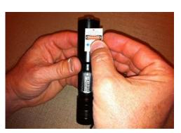
11. Fill out and apply the laser warning label to the heat sink holder, slightly overlapping the battery compartment if necessary. "Max power" is 1,500mW, "Wavelength" is 445nm, "Voltage" is 4.4, "Class" is IV, "Pattern" is Point. **Note:** The red arrowhead on the label points toward the lens. Your laser is now completely assembled and ready for use.
