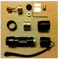
2. Remove and unpack all parts from the bundle and **completely** parts disassemble the laser host into the five major components shown. Verify that all parts are included in the bundle. L-**R**: diode & driver module, lens cap, lens focusing ring, laser warning label, 0.050" Allen wrench, AR coated glass lens (may assembly be wrapped), bezel/retaining ring, heat sink w/set screw, heat sink holder, battery compartment, tailcap w/switch and wrist strap. Note: Lens spring not shown in photo.
